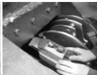
removing of the knives for sharpening
